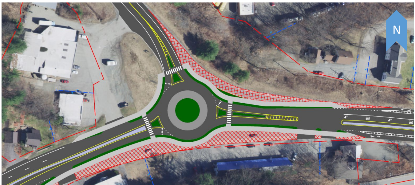
Figure 12. Alternative #5 Intersection Layout.
